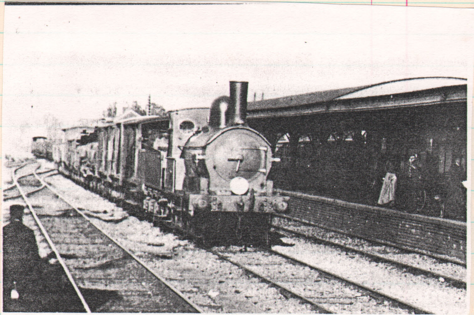
Andover Junction 16/9/1899 Single-framed Boyer 0-6-0 No. 373 (Built 1878) on up goods. Headcode; West of England - Nine Elms fast goods
